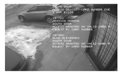
13. Once the text overlay is properly configured on both sides (SRX-Pro and Portal), the operator may start using the camera icon that accompanies each event in the Portal Log Monitor. On double-click, the DVMS will open the corresponding video channel in the SRX-Pro Search mode. The exact moment of the event occurrence will be displayed in the search mode.
