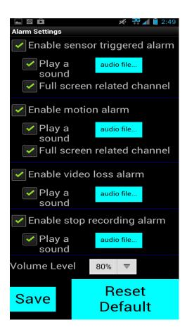
**Enable sensor triggered alarm**. Tick the checkbox to enable an alert whenever a Sensor alarm has been triggered on a connected remote Server.
