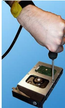
Place the bay with the inserted hard drive flat on a clean, leveled and stable surface. Locate four (4) small bay screws (inside the plastic bag taped to the front panel of your unit). With the Philips screwdriver screw the hard drive to the hard drive bay as shown on the picture.
