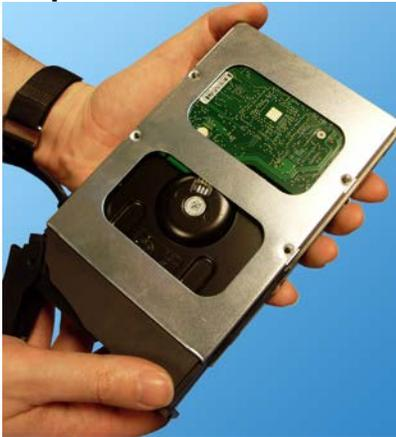
Slide the new hard drive inside the provided hard drive bay as shown on the picture. The hard drive circuitry should remain exposed (see image).
