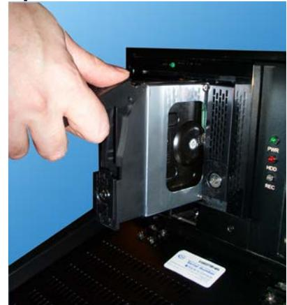
Slide the hard drive bay with the new hard drive inside the hard drive bay slot. Push the top portion of the bay into place to lock the bay into the SATA enclosure box. Use the SATA keys provided (tie-wrapped to the back of the unit) and lock all bays that contain hard drives. Repeat all above steps for all additional drives. Connect the power to the unit and power up the HVR/NVR.
