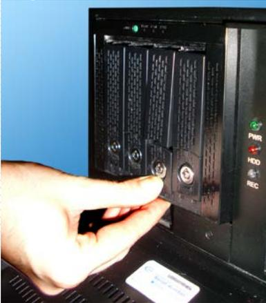
Once the empty bays are unlocked, place your thumb on the lower portion of the empty bay and push it downwards, this will make the bay come forward and the upper portion of the bay to elevate.
