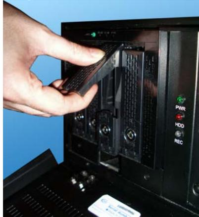
Firmly hold the top portion of the hard drive bay and pull the bay forward.
