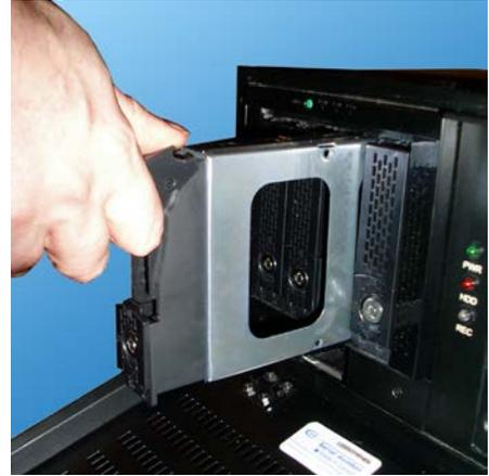
The empty hard drive bay will slide out of the SATA enclosure. Remove the bay from the enclosure.
