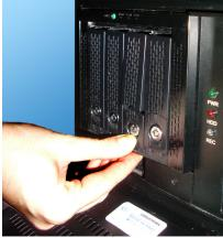
Shut down the DVR and unplug the power. Open the unit door and locate the SATA hard drive enclosure.
