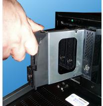
The empty hard drive bay will slide out of the SATA enclosure. Remove the bay from the enclosure.
