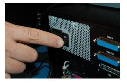
Switch the power switch on the Power Supply to the OFF position.
