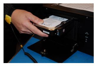
Use the plastic key included in your accessories box or a pointed object, such as a screwdriver or a pen to unlock one of the top two hard drive bays. Push the sliding tab to the bottom, covering the red dot. The bay will be unlocked.
