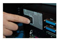
Switch the power switch on the Power Supply to the OFF position.
