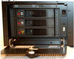
Open the unit door and locate the hard drive bay. All three hard drive slots should be locked. This is indicated by the red dot on each respective HDD slot.
