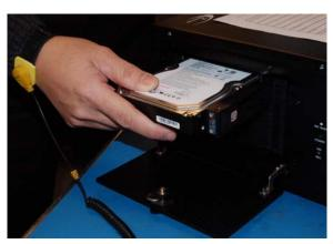
Position the new hard drive face up and with the connectors facing away from you and to the inside of the DVR unit.
