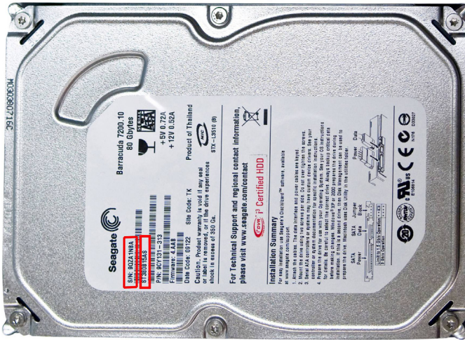
Picture 1. Serial Number of the Seagate hard drive is located directly beneath the Seagate logo in the top left corner. The hard drive model is printed below the serial number.
