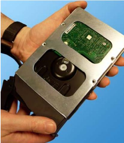
**Ground yourself** and slide the new hard drive inside the provided hard drive bay as shown on the picture. The hard drive circuitry should remain exposed (see image).
