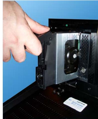
Slide the hard drive bay with the new hard drive inside the hard drive bay slot. Push the top portion of the bay into place to lock the bay into the SATA enclosure box.
