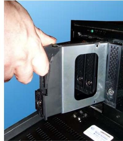
The empty hard drive bay will slide out of the SATA enclosure. Remove the bay from the enclosure.
