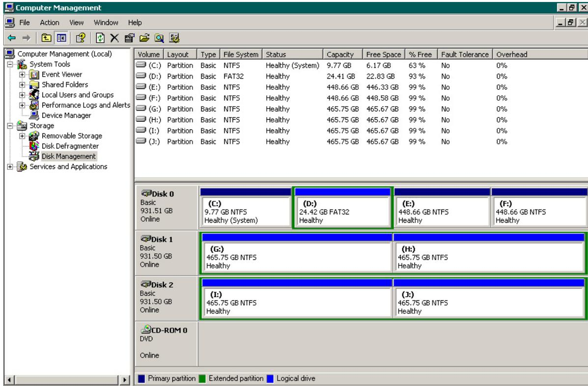
This completes the new hard drive configuration. Restart SRX-Pro Server, go to Setup -> Storage Setup and allocate all new partitions for video recording.
