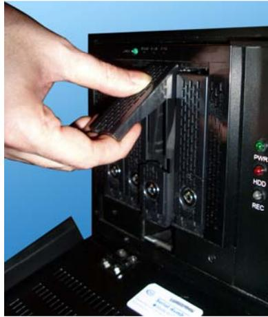
Firmly hold the top portion of the hard drive bay and pull the bay forward.
