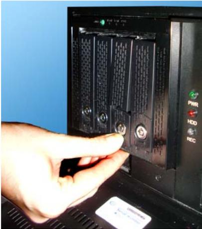
Shut down the DVR and unplug the power. Open the unit door and locate the SATA hard drive enclosure.
