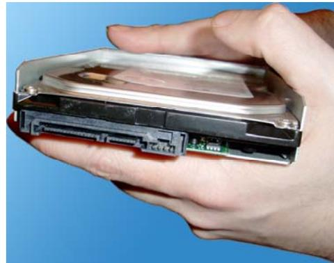
The hard drive must be positioned in the bay in such a way that the drive connectors are exposed and face away from the closed side of the bay.
