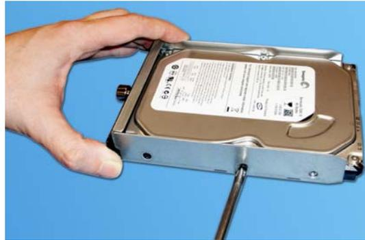
Place the bay with the inserted hard drive flat on a clean, leveled and stable surface. Locate six (6) small bay screws (shipped separately inside the accessory box). With the Philips screwdriver screw the hard drive to the hard drive bay, 3 screws on each side.
