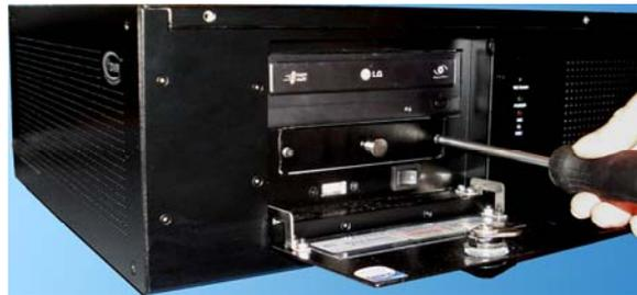
Using the Philips screwdriver, re-attach the hard drive bay to the unit with 2 screws.
