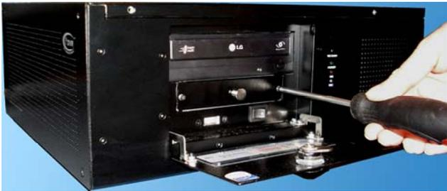
Shut down the DVR and unplug the power. Open the unit door and locate the hard drive bay. Using the Philips screw driver remove two screws that hold the hard drive bay in place.
