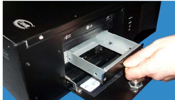
Hold onto the provided bay handle and pull the empty hard drive bay out. Remove the empty bay from the unit.
