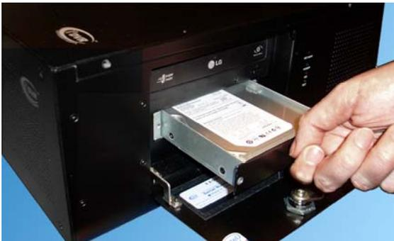
Slide the hard drive bay with the new hard drive inside the hard drive bay slot.
